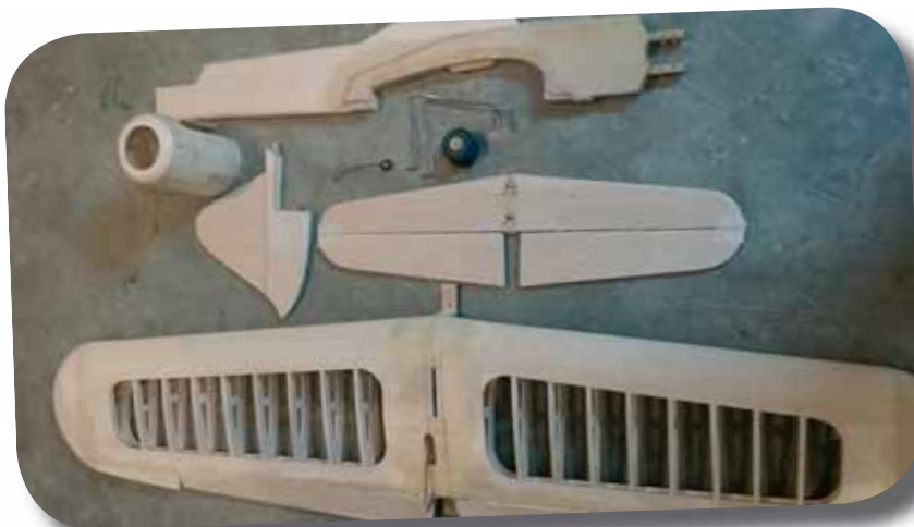
All woodwork finished. This is what the model looks disassembled. The wing is made in one piece and cannot be taken apart.
