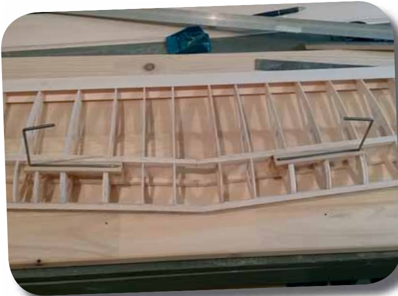
Hardwood reinforcements are made for the landing gear and supported by the wing construction. As a last step most of the wing is covered with thin balsa sheets.
