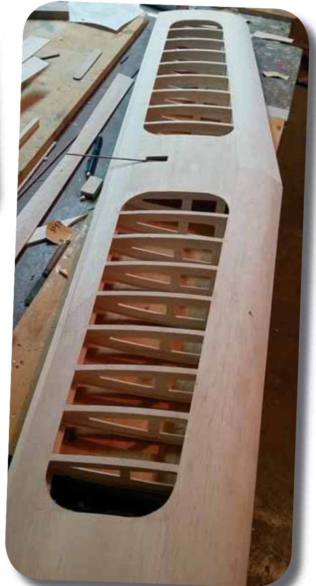
The wing have a traditional construction with moldings and balsa ribs.
