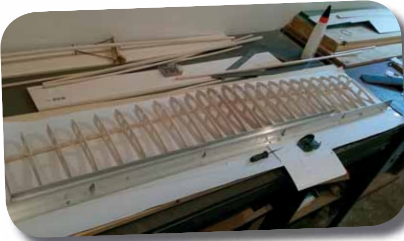
The wing have a traditional construction with moldings and balsa ribs.
